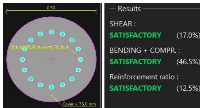
Figure 4.42. Reinforcement of pile under Interior column
