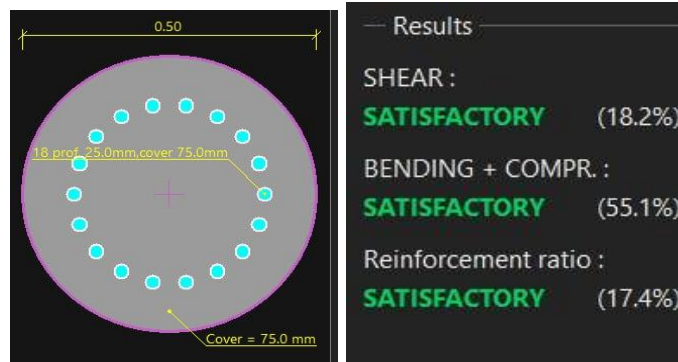
Figure 4.44. Reinforcement of pile under Corner column
