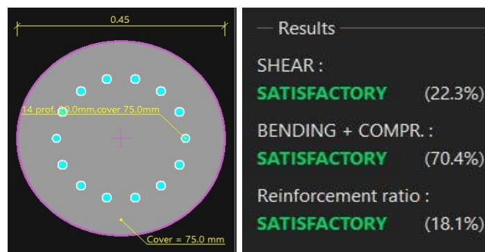
Figure 4.43. Reinforcement of pile under Exterior column
