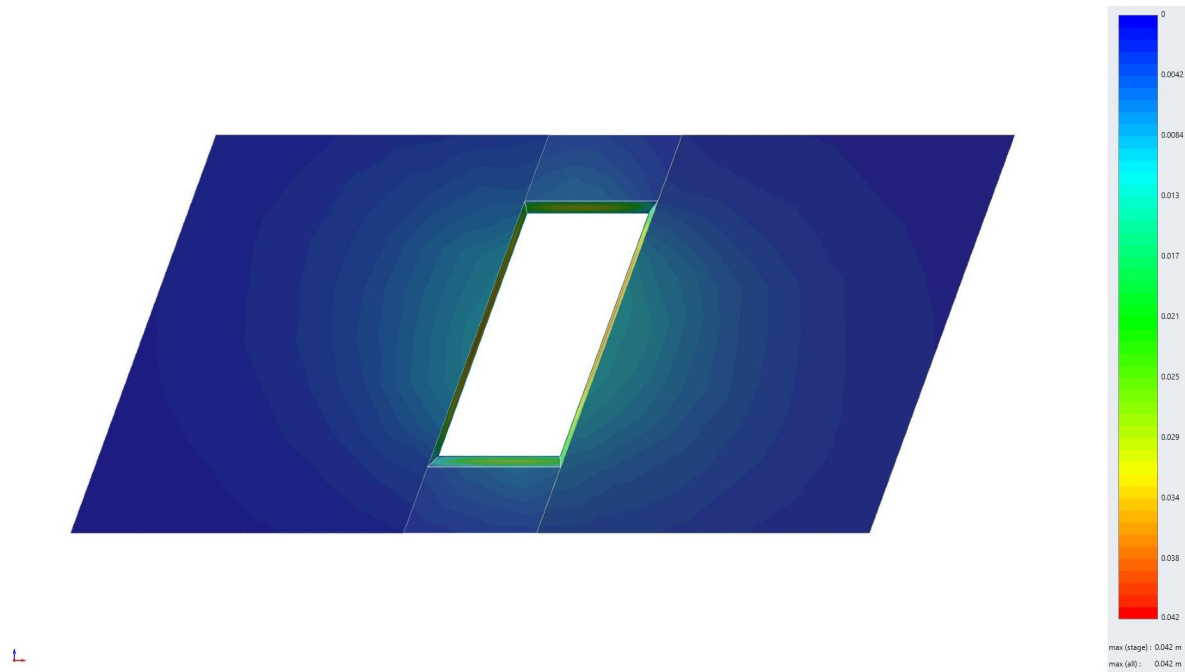
Figure 29. 3D simulation result representing total displacement after the stope excavation.
