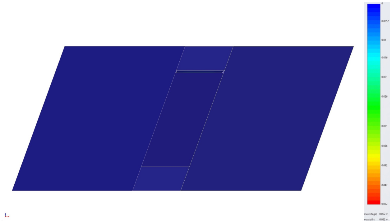
Figure 35. 3D simulation result representing total displacement after the backfilling.
