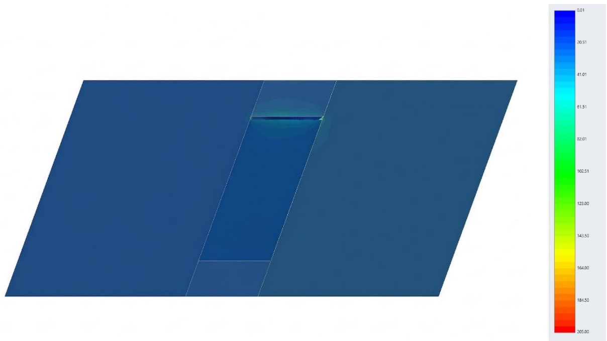
Figure 36. 3D simulation result representing major principal stress ( \sigma_1 ) after the CO 2 injection.
