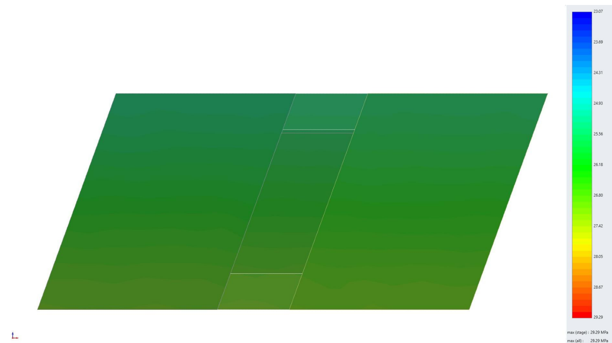
Figure 25. 3D simulation result representing major principal stress ( \sigma_1 ) at virgin state.
