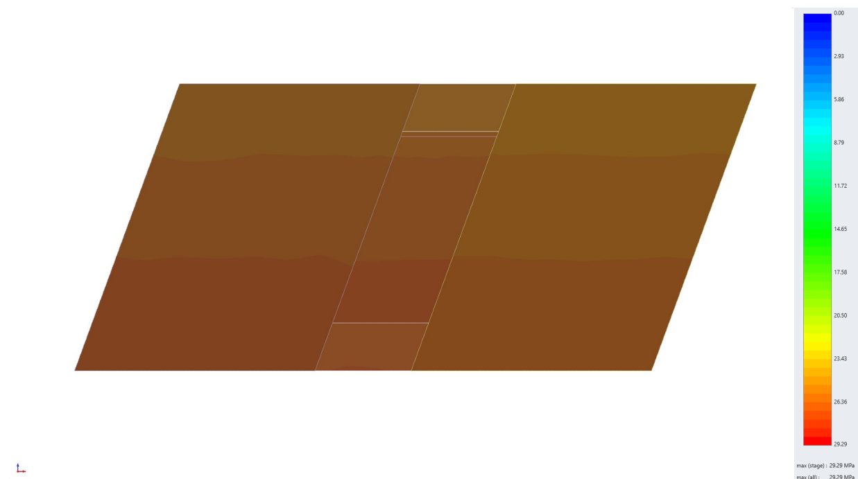
Figure 26. 3D simulation result representing minor principal stress ( \sigma_3 ) at virgin state.
