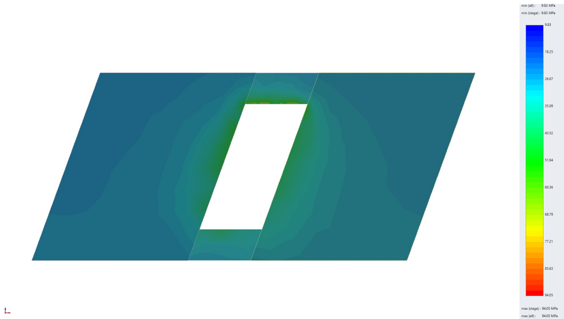
Figure 27. 3D simulation result representing major principal stress ( \sigma_1 ) after the stope excavation.
