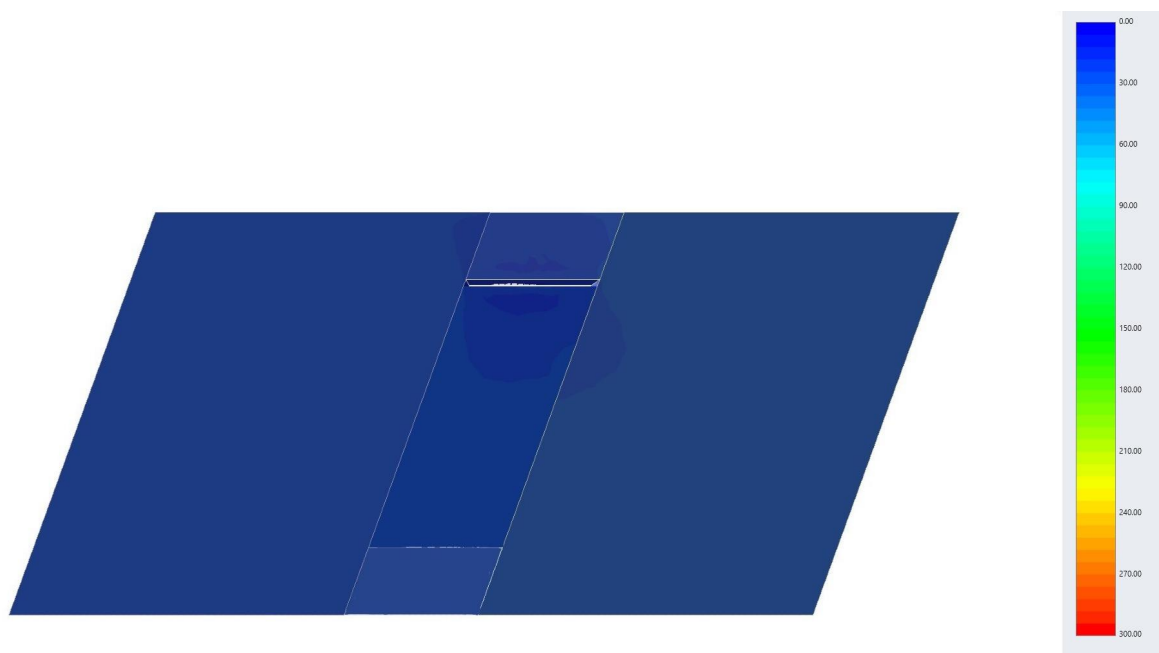
Figure 37. 3D simulation result representing major principal stress ( \sigma_3 ) after the CO 2 injection.
