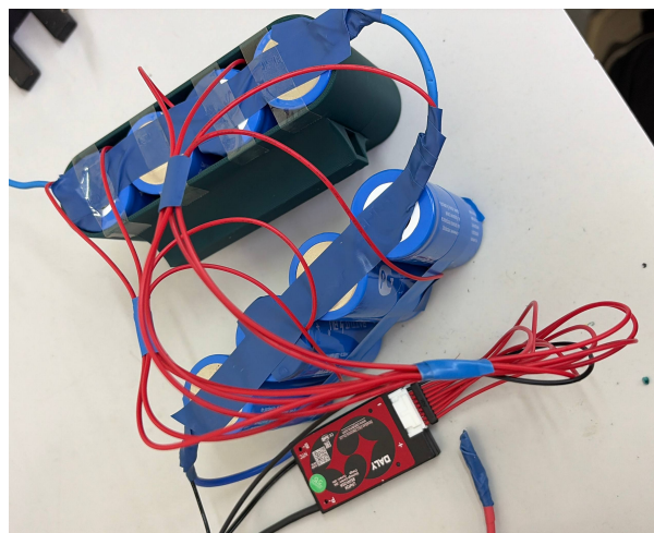
Figure 7.8: Custom 8S1P LiFePO4 battery assembly with integrated Daly BMS.
