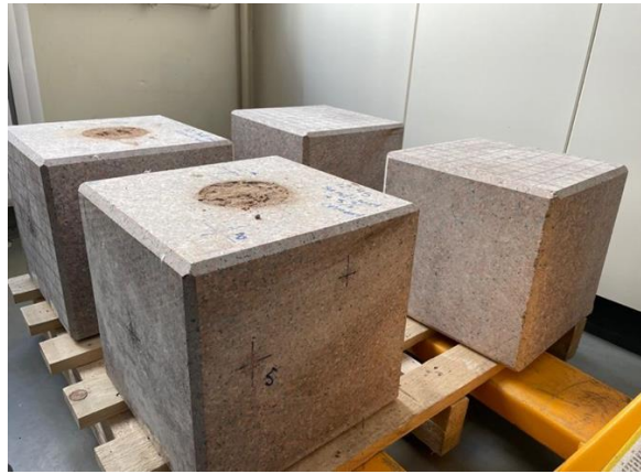
Figure 4. Granite rock samples with the cube size 300 mm with and without holes (hole diameter is 100 mm)
