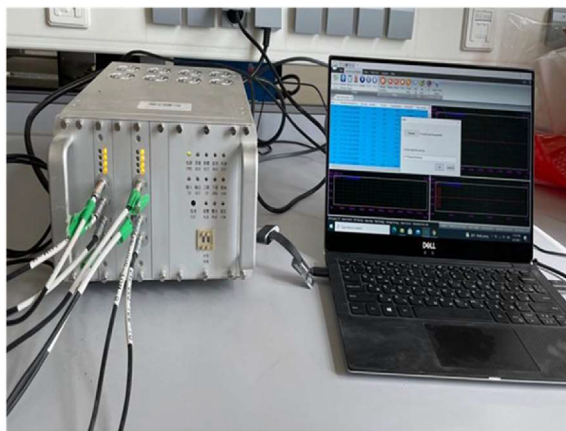
(a) AE data acquisition modules, chassis with front and rear panels, optional network communication module, laptop
