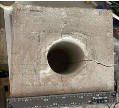
Figure 1. Fractured cube with 3 joints.
