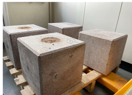
Fig. 2. Granite rock samples with a cube size of 300 mm with and without holes (hole diameter is 100 mm).
