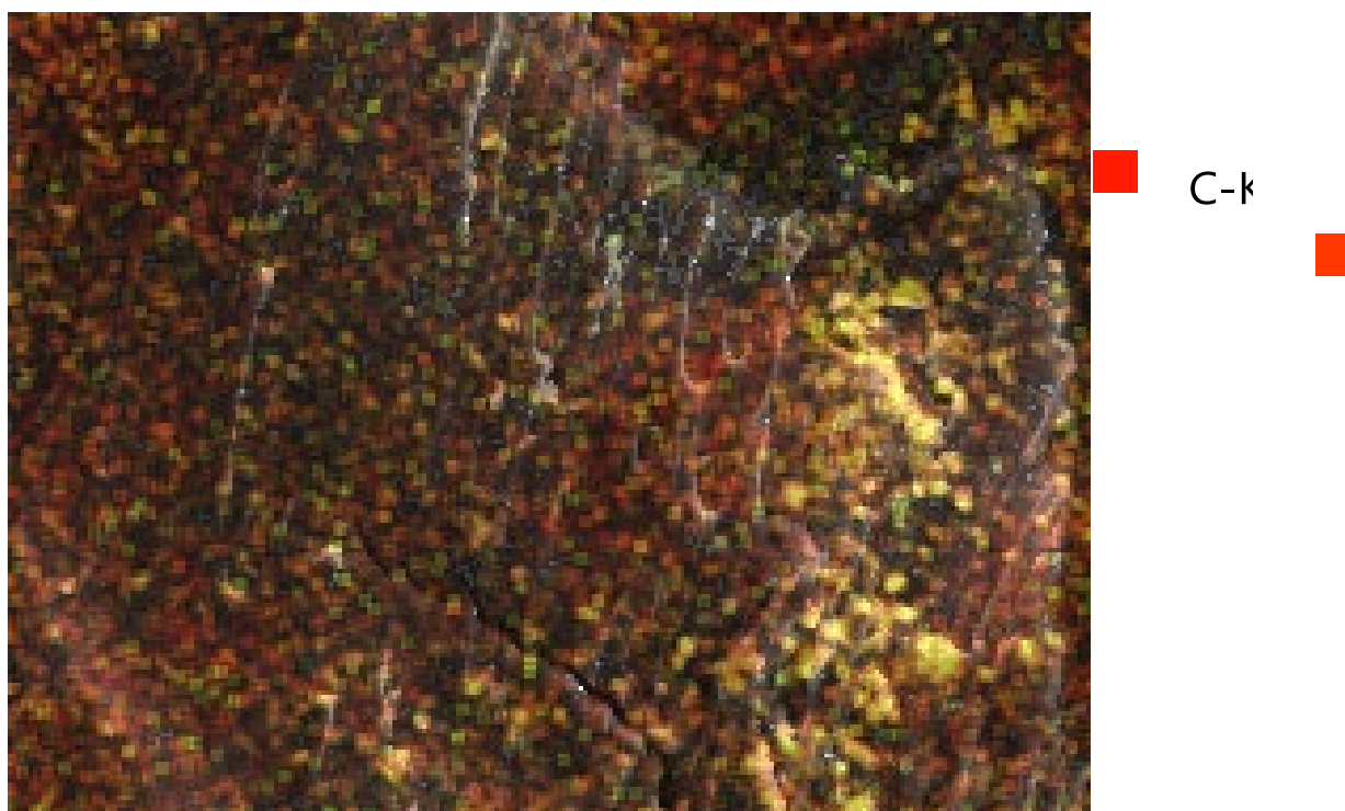
Figure 5-19. Map of local elements by EDS analysis for asphaltene sample #3
