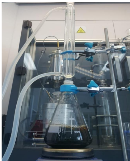
Figure 4-4. Boiling the mixture of crude oil and n-heptane under the reflux
