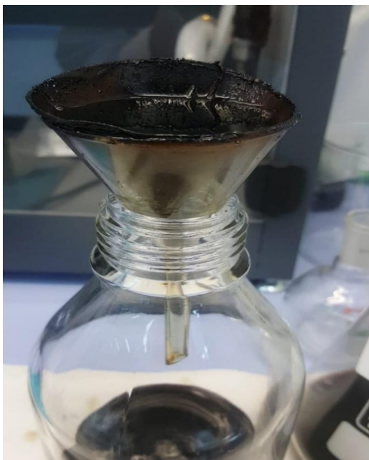
Figure 4-3. Filtration of asphaltenes
