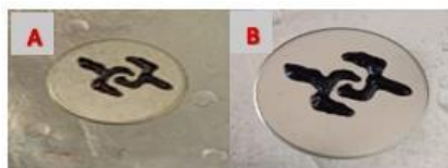
Figure 1. Illustrate different 3D printed electrodes with different proportions and printing pressure (a) 80:10:10/108kPa, (b) 70:15:15/120kPa.
