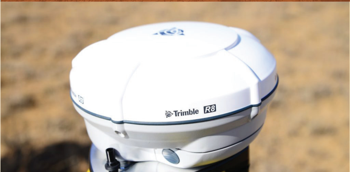
Multifunctional high-precision GPS multsystem / GLONASS receiver
