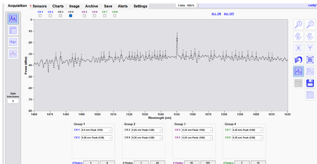
Figure 3.3: Example of spectrum of the sensor with high sensitivity
