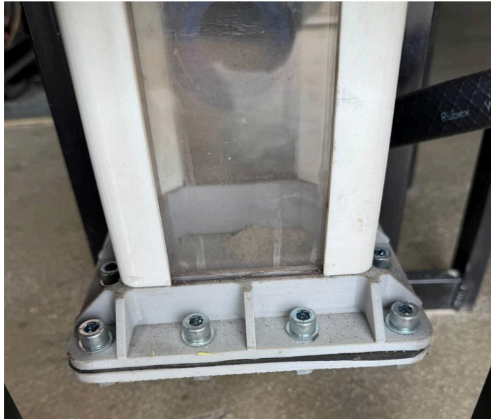
Figure 44. Sand leakage to the air plenum of AR.
