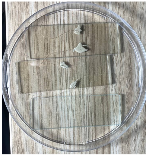
(a) 50 nm thin ITO deposited glasses with copper wires, next to a regular glass
