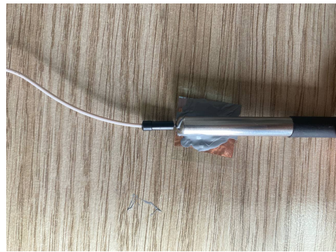
(b) DS18B20 sensor mounted to ITO-glass via thermal paste)
