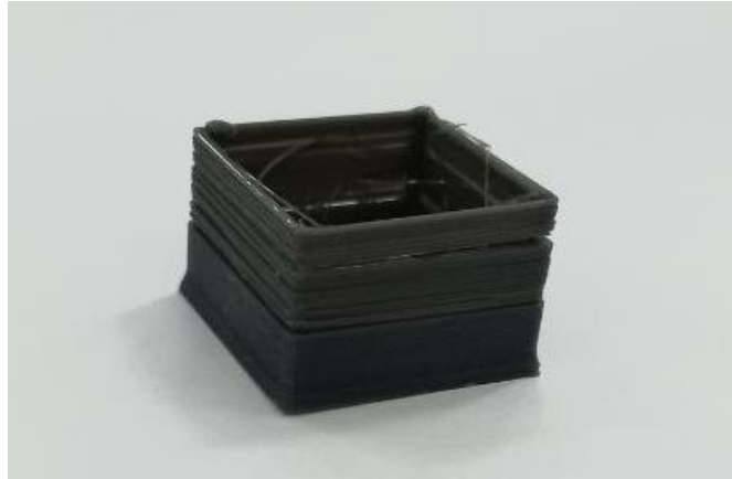
Figure 6: Printed part with under extrusion
