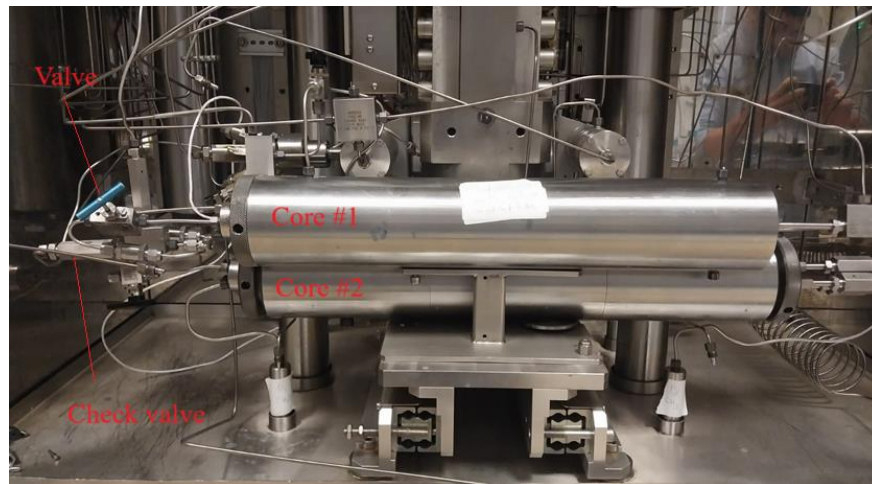
Figure 3-8. Dual core holder system.
