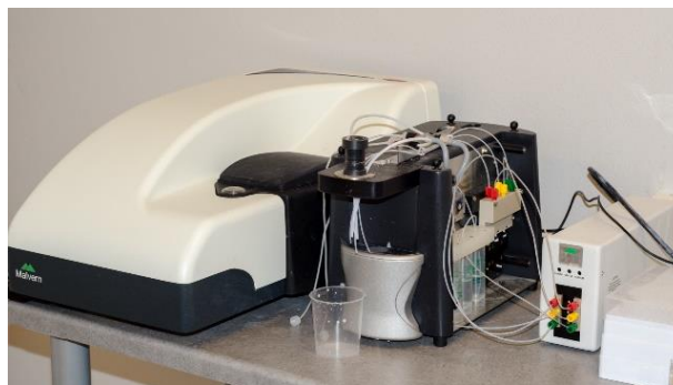
Figure 3-5. Zetasizer Nano ZS system used in this study.
