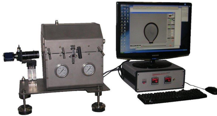
Figure 3-9. HPHT Interfacial Tension Meter (IFT 700).
