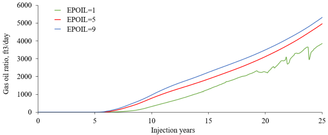
Figure 5-18. Gas-oil ratio at various epoil values.
