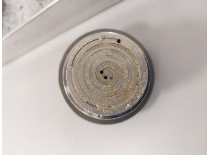
Figure 4-2. The surface of inlet plug of the core-holder.
