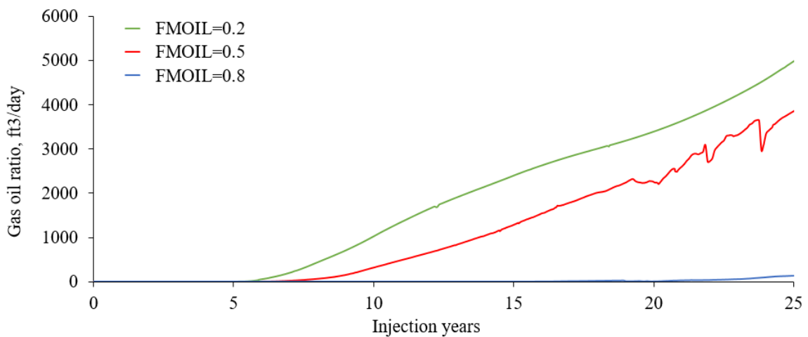
Figure 5-16. Gas-oil ratio at various fmoil values.
