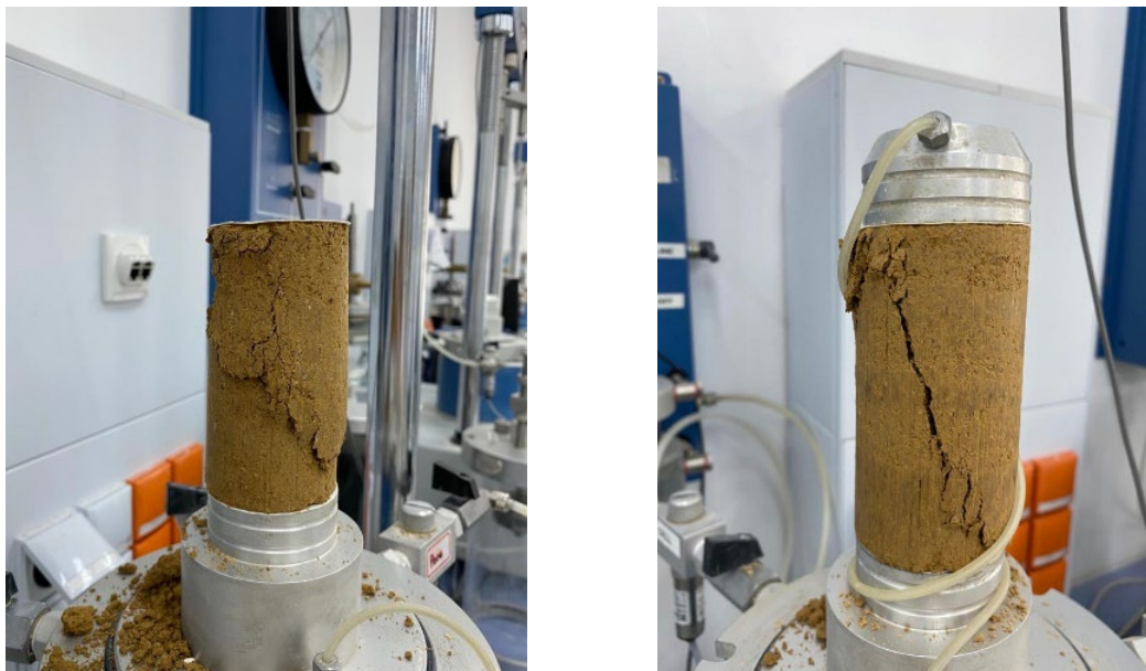
Figure 4.4: Failure planes of soil samples treated with CSA cement
