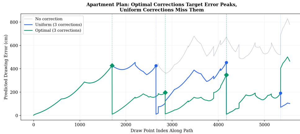
Figure 4-4: Apartment plan- predicted error along the drawing path. Optimal correction points of Green diamonds coincide with peak errors; Uniform points of Blue circles sometimes appear at the low error position, hence, correction opportunities are not utilized efficiently.
