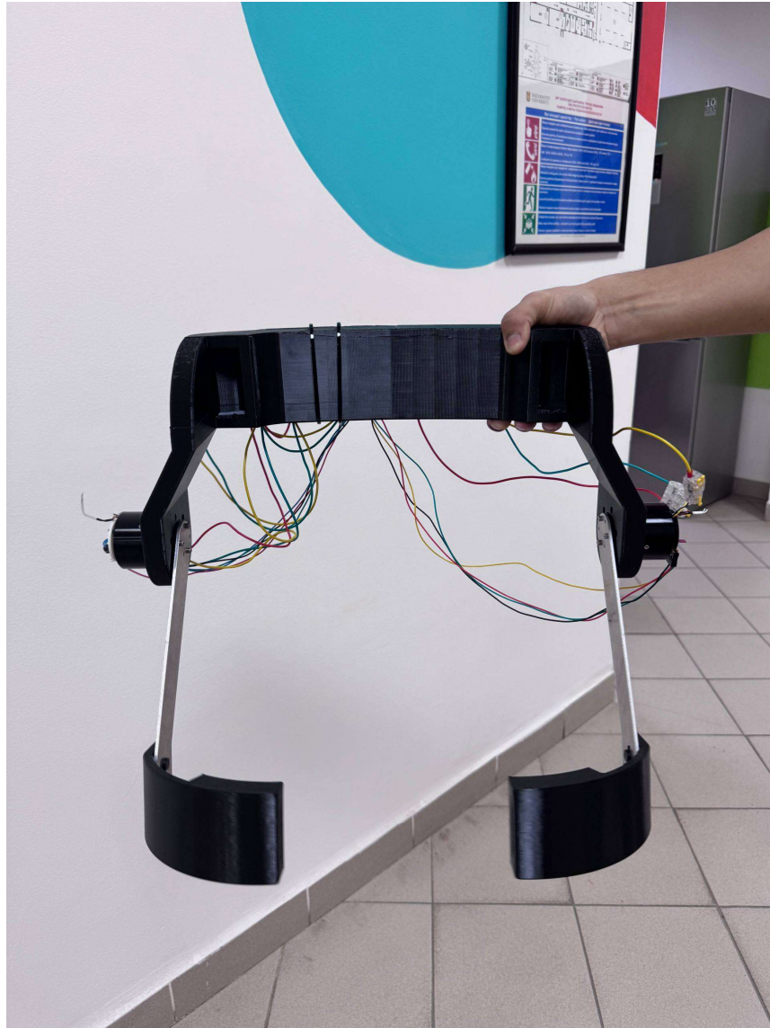
Figure 3.2. Assembled hardware prototype of the bilateral wearable hip exoskeleton. The prototype comprises the 3D-printed PLA pelvic frame, bilateral lateral uprights, CubeMars AK45-10 actuation modules mounted at each hip joint, thigh cuff interfaces, and the ODrive v3.6 motor controller with associated wiring. The internal driver boards of the AK45-10 actuators are bypassed, with the three-phase stator leads and magnetic encoder connectors routed directly to the ODrive controller as described in Section 3.1.4. Full closed-loop commissioning of the assembled prototype is planned as Phase 1 of future work (Section 5.2.1).
