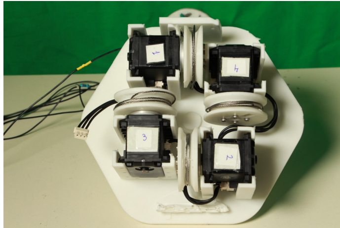
Figure 3.1.1: Four Dynamixel MX-28 servos are used to actuation plate, which provide independently tension to the left, right, up, and down tendons.
