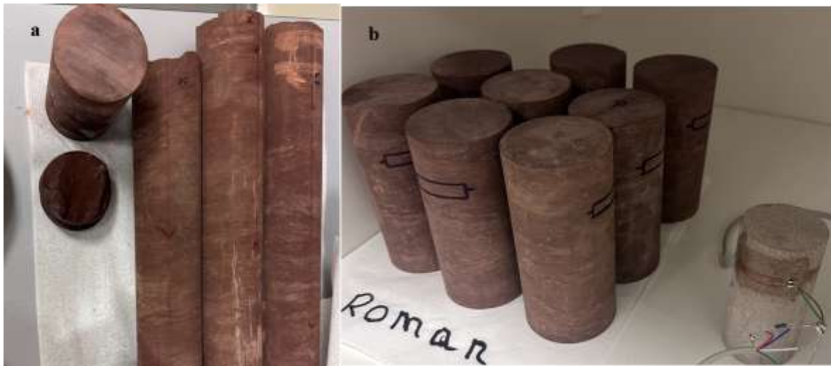
Figure 4.1 Example of rock sample preparation for the test: a) example of delivered cores, b) prepared rock samples for UCS test
