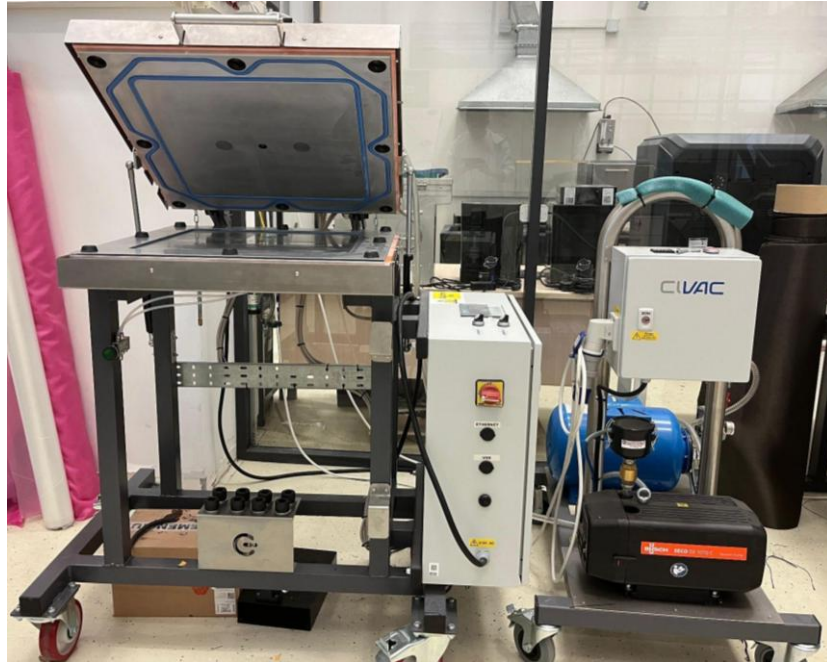
Figure 7. Vacuum assisted resin transfer machine.
