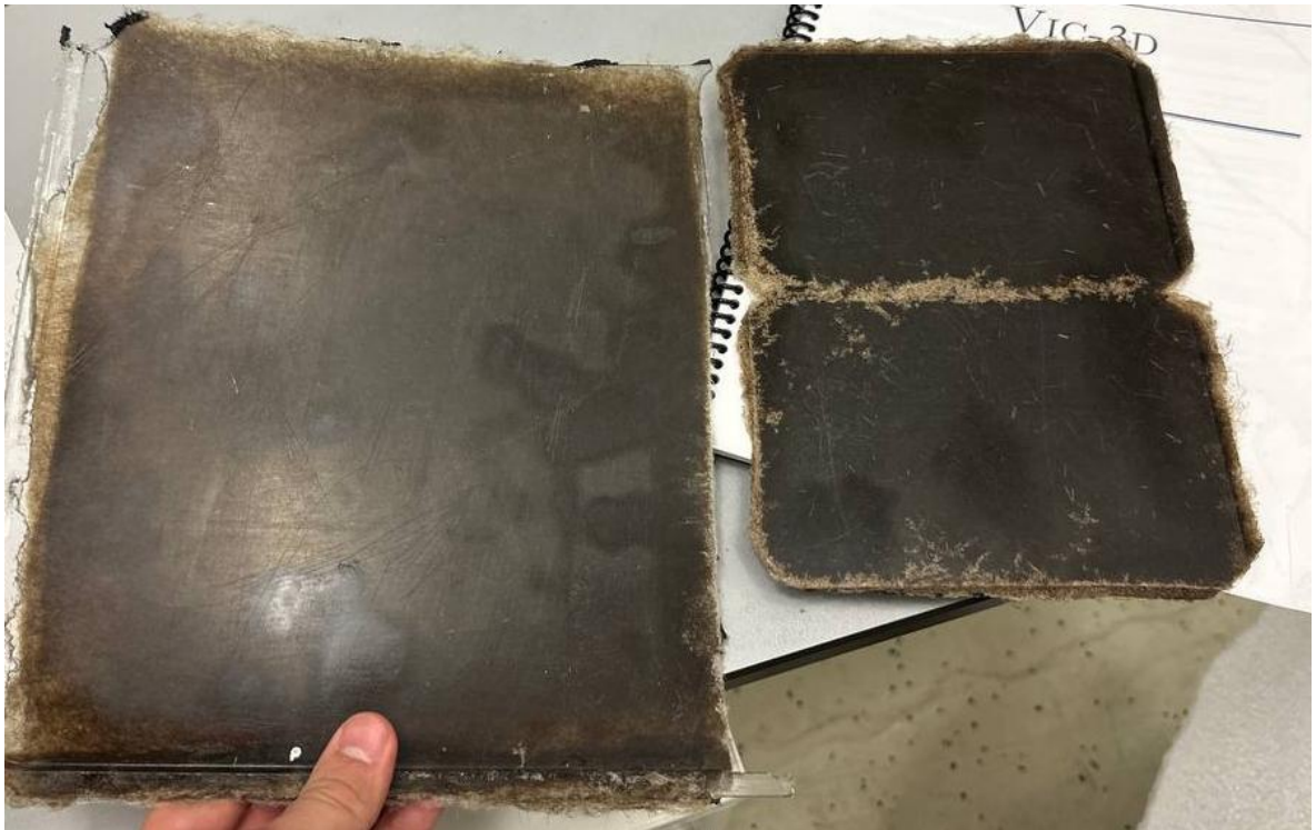
Figure 45. Fabricated fiber-epoxy composite with addition of date seed derived particles prepared for tests.
