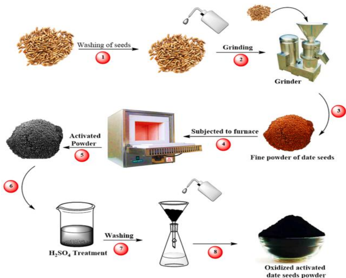
Figure 42. Illustration of the complete formation of OACDS. [27]
