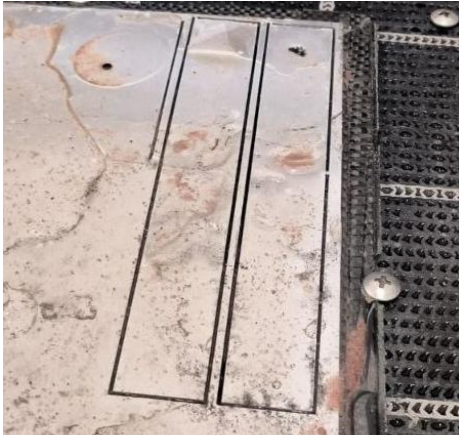
Figure 20. FML panel during water jet cutting.
