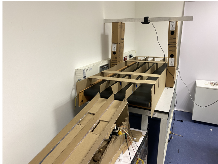
Figure 4.2: Final potato sorting system setup, showing conveyor, camera, and divider arrangement
