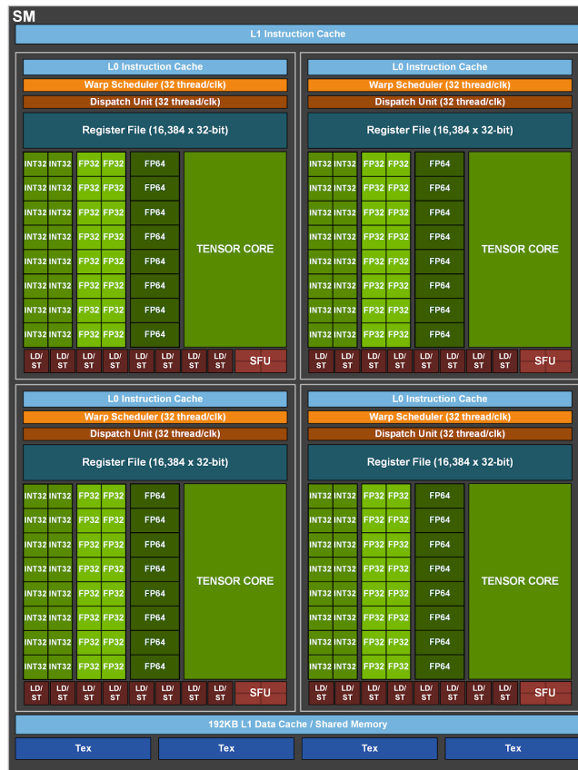
Figure 1.2: Streaming Multiprocessors (SM) are the main elements of parallel computations, where many CUDA cores are utilized for high-throughput, floating-point performance. Each SM possesses a multilevel memory hierarchy: private registers assigned to every single thread, shared memory used by all threads within one block, and global memory for data storage of a wider scope. A warp scheduler manages the execution of 32-thread groups called warps and ensures that all threads execute the same instructions at every clock cycle in lockstep (source image: Nvidia).
