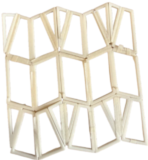
Figure 5.3: Unfolded state of origami structure .
