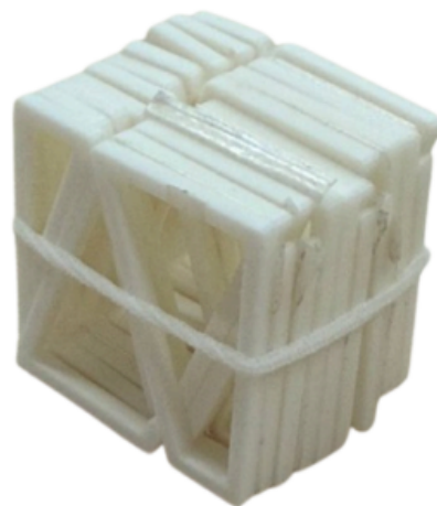
Figure 5.4: Folded state of origami structure
