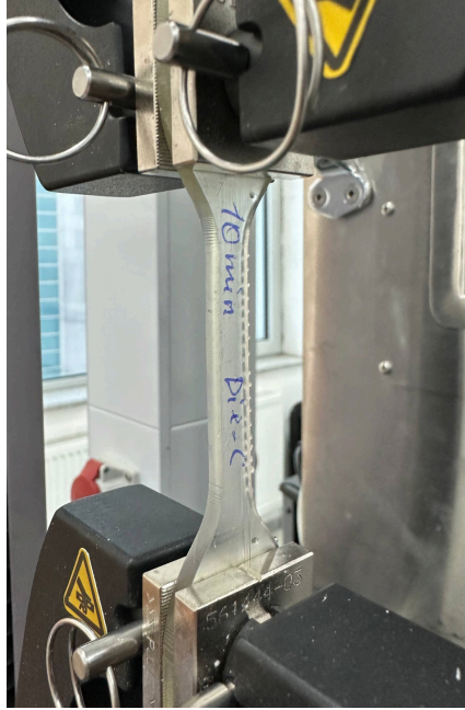
Figure 30. Fixing specimen (10 min. curing-time)
