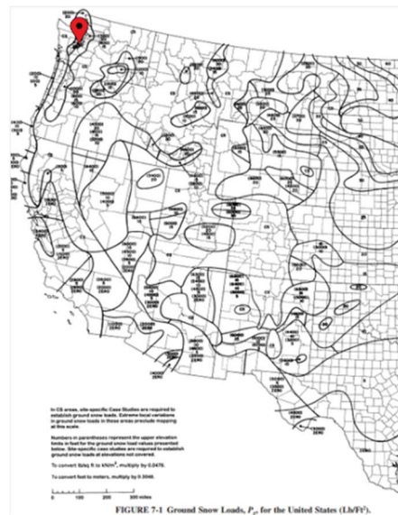
Figure 4.1. Ground Snow Loads for USA
