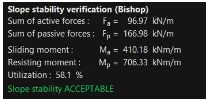
Figure 5.23. Slope stability analysis in Geo5
