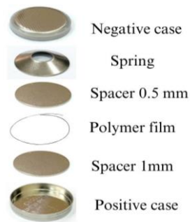
Figure 14. Schematic representation of coin cell assembling for PEIS analysis.
