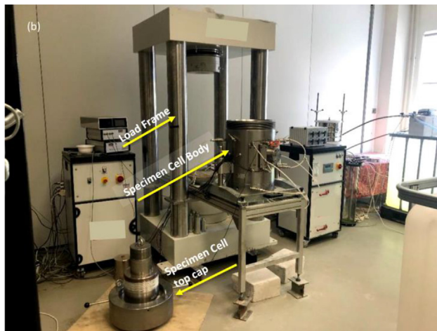
Fig. 2. High pressure consolidation system: (a) Schematic diagram, (b) General view, and (c) Specimen cell in the loading position.
