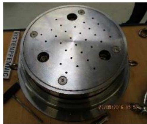
Fig. 6. Bottom plate of high pressure consolidation cell: (left) Bottom and (right) Top views.
