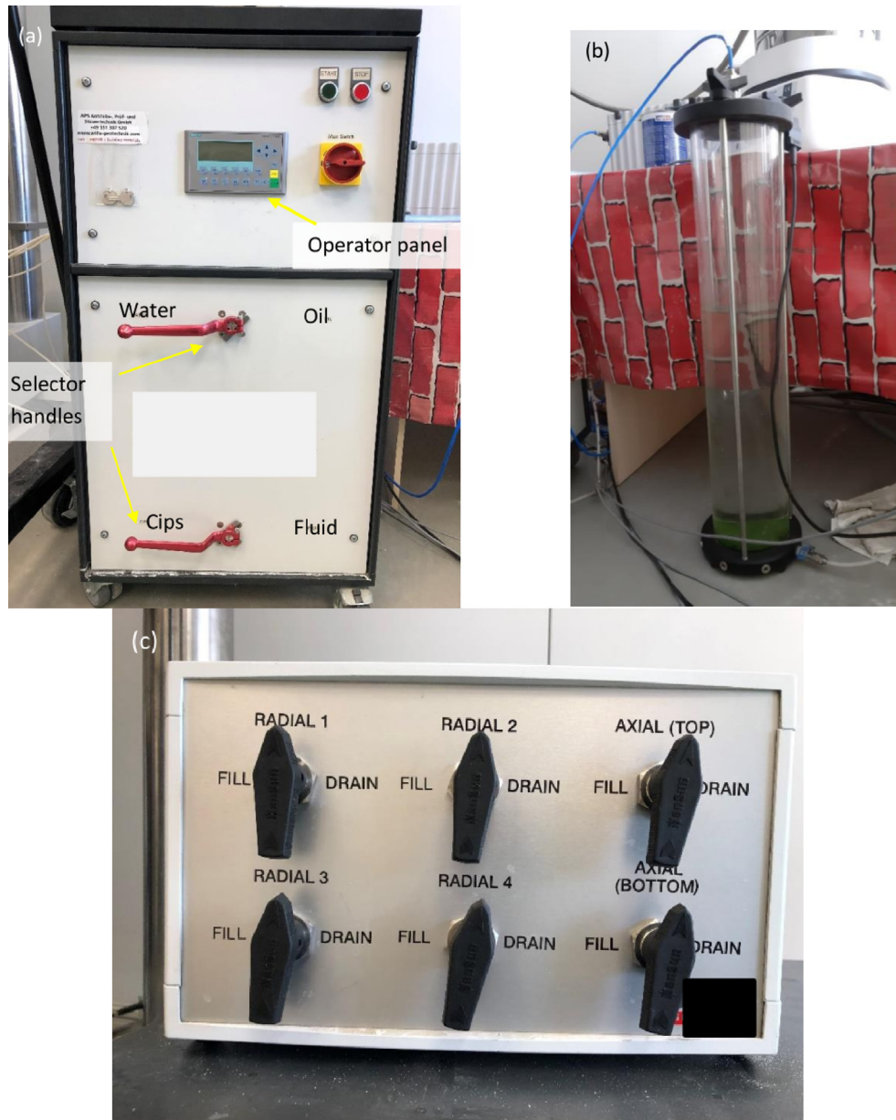
Fig. 8. Liquid supply system: (a) Multiphase pump unit, (b) Air/liquid pressure cylinder, and (c) Valve operation unit.
