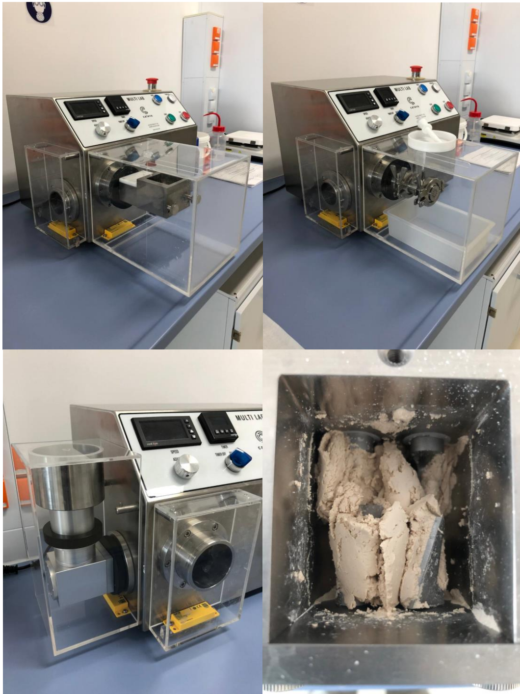
Figure 1: Caleva Multi Lab equipment with interchangeable mixing/kneading, extrusion, and spherization parts. The last image shows the prepared paste for extrusion.
