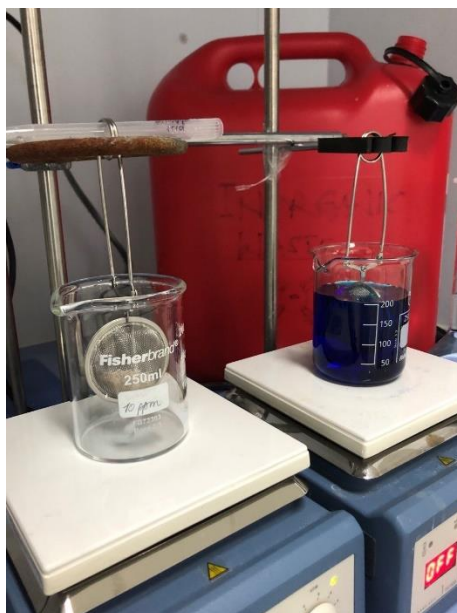
Figure 4: The experimental setup of the methylene blue adsorption experiments with kaolin pellets.
