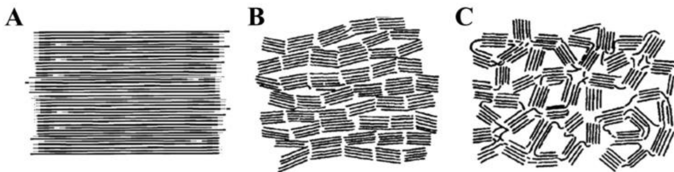
Figure 2. Schematic illustration of structure of a) graphite, b) soft carbon, c) hard carbon [29].
