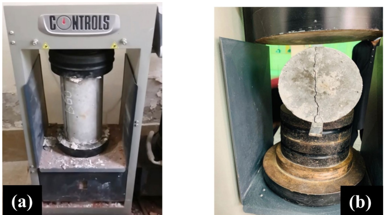
Fig. 2. Laboratory testing (a) CS testing and failure plan, and (b) TS testing and failure plan.
