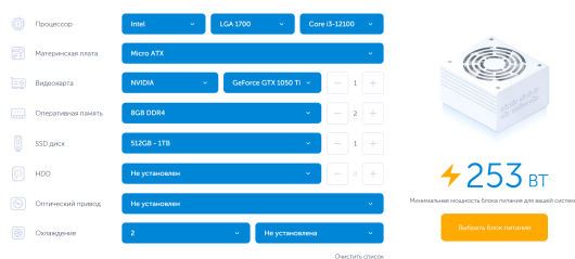
Fig. 1. Calculated minimum power usage for a GPU-based car plate recognition computer. ( https://shop.kz/calculator-moschnosti-bloka-pitaniya/ )
