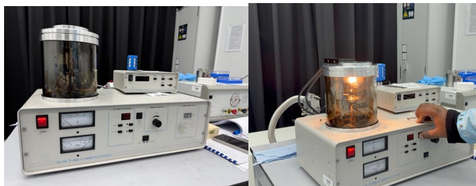
Fig 10. Sputter Machine for carbon coating
