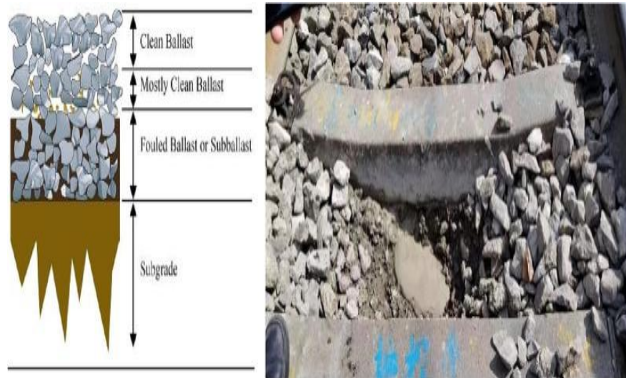
Figure 2-8. Particle layer fouling (C. Shi et al., 2023b)
