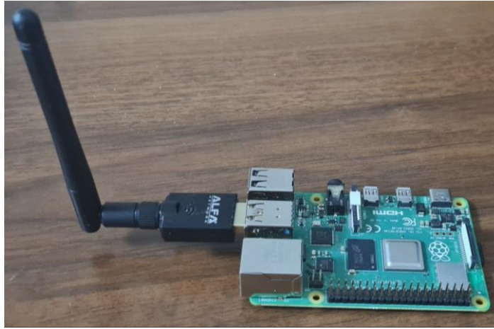
Figure-8.1.1. RX side of the design. Raspberry Pi 4 Model B equipped with the Alfa Network AWUS036ACS Wi-Fi transceiver. Mounted on an UAV during the experiment alongside a power supply. The SD card is inserted in the Pi beforehand and serves as Raspberry Pi OS (Raspbian) repository in which the software design can be implemented
