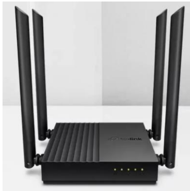
Figure 8.1.2. TX side of the design. TP-Link Archer A64 is a conventional Wi-Fi router. It is used as the transmitter of the Wi-Fi packets, also known as beacons. Thus, the router may or may not be left as an idle device by not connecting to any existing network. Either way, the beacons will always be present in the Wi-Fi packet transmission.
