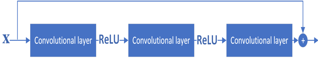
Figure 4-2: Residual block implementation. Adapted from [28]
