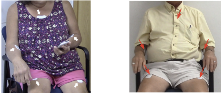
Figure 2-2: Multi-sensor wearable setup for PD monitoring, with sensors placed on arms, legs, and chest. Adapted from [11, 3].
