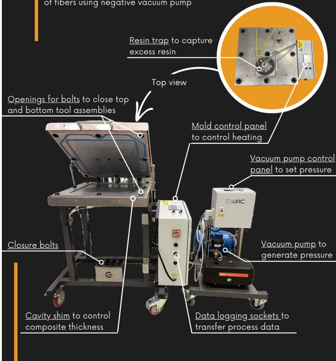
Figure 4. Vacuum assisted resin transfer mold
