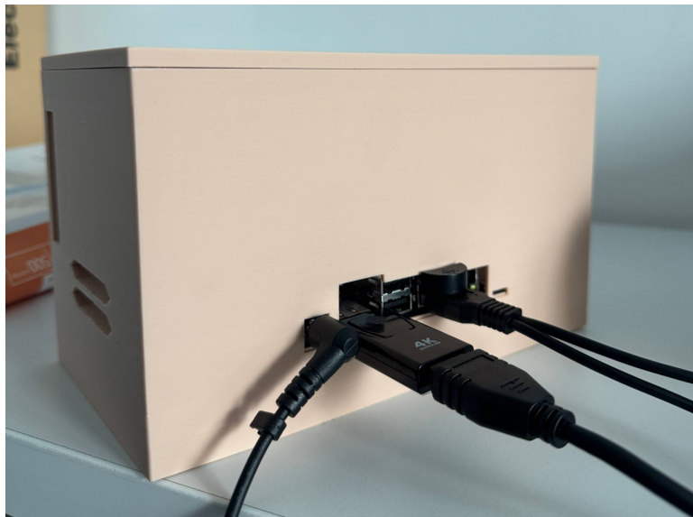
Fig. 8. Rear view of the Boxy enclosure showing the Jetson Orin Nano module, power supply connector, DisplayPort, microphone USB, and display USB cutouts on the back panel.
