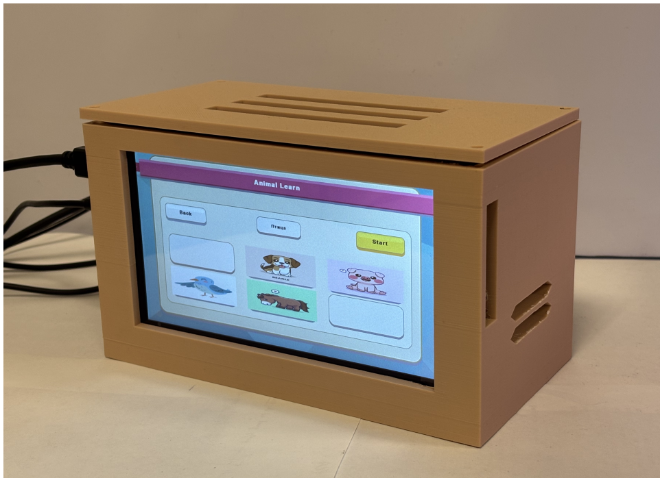
Fig. 7. Fully assembled Boxy device showing the front view: LCD touchscreen displaying the Animal game, with the NVIDIA Jetson Orin Nano, USB microphone, and speaker.
