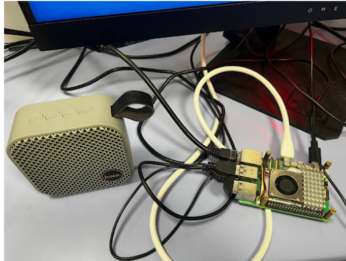
Fig. 9. Fall 2025 prototype: Raspberry Pi 5 thin client with USB microphone and portable speaker, used as the initial audio I/O device before migration to the Jetson Orin Nano.
