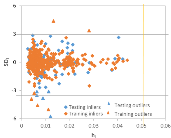
Figure 16. William's plot for the training and testing datasets of the CMIS model.
