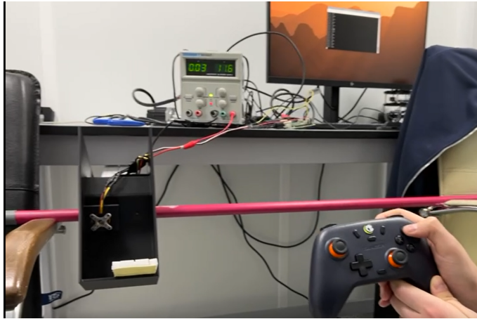
(a) Validation setup for Iteration 3.5: Testing on a horizontal tube using a GameSir controller and DC power supply.
