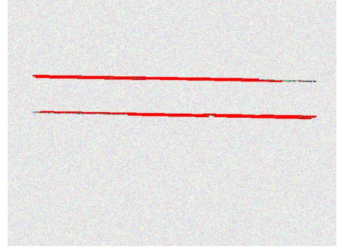
(b) Hough output on synthetic image: both conductor lines correctly identified (red overlay).
