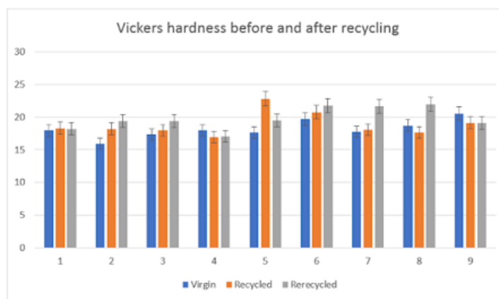
Figure 3.20: Comparison of Vickers hardness values for virgin, recycled and re-recycled PLA
