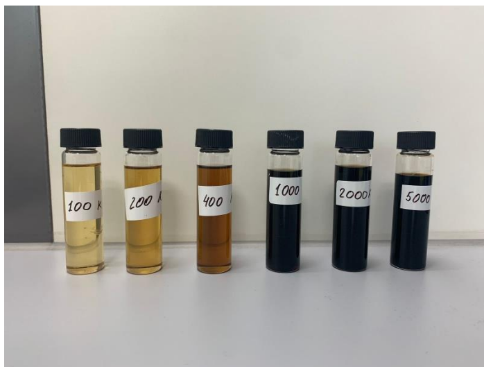
Figure 3-5. Supernatant liquid after centrifugation of TGA samples.
