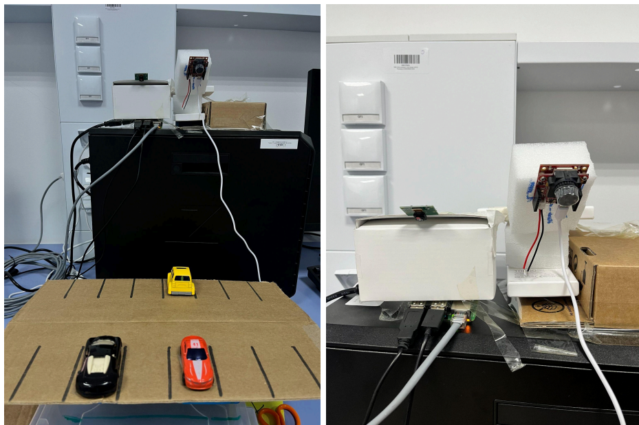
Figure 12. Full hardware setup with toy parking setting. Devices: Pi Camera the on left and OpenMV Cam H7 the on right.
