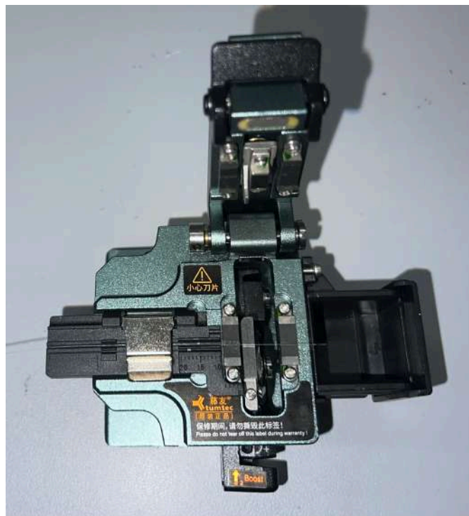
Image 1. A demonstration of SMF ready to be cleaved and cut by the cleaver
