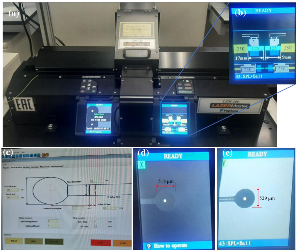
Figure 2. 1: Fabrication of OFBR (a) Fujikura LZM-100 Splicer, (b) inset image of optical fibers layout, (c) Ball resonator Set parameters, (d) and (e) Image of the ball resonator showing x and y diameters.
