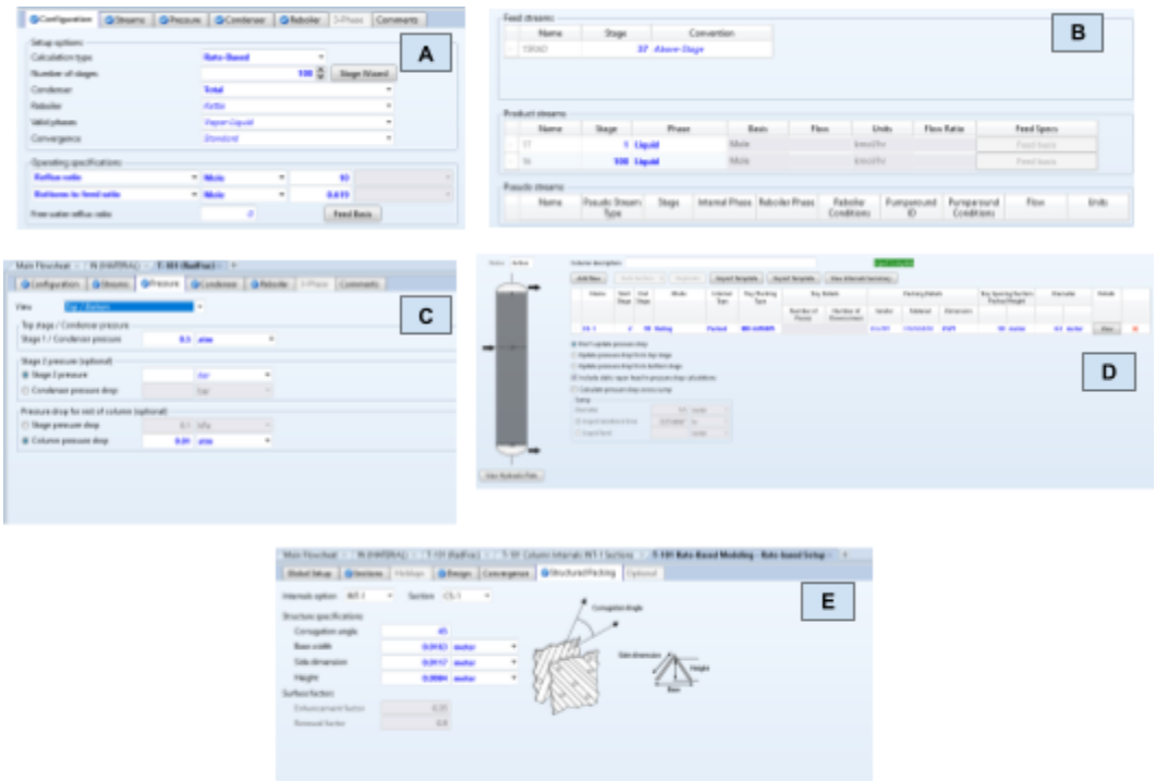
Figure J3. Input to RadFrac: (A) Configuration, (B) Streams, (C) Pressure, (D) Design and internal specifications, (E) Geometry of packing material
