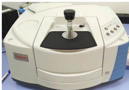
Figure 3-7. Nicolet iS10 FT-IR Spectrometer.
