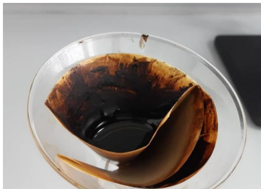
Figure 3-4. Filtration process of asphaltene precipitate.
