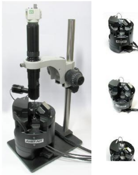
Figure 3-11. The AFM System – SmartSPM 1000.
