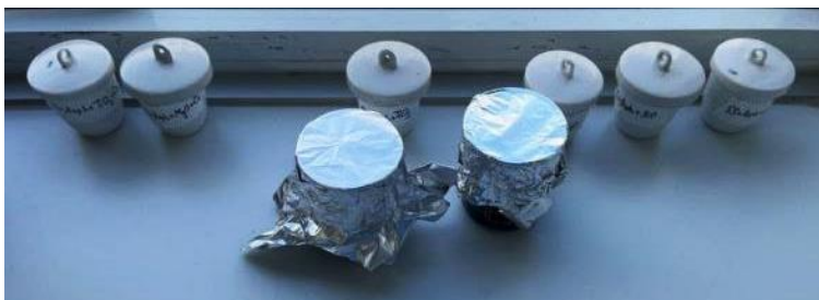
Figure 3-14. The samples prepared for investigation of asphaltene adsorption.
