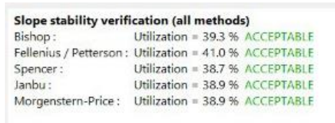
Figure 70. Slope stability of the sheet pile
