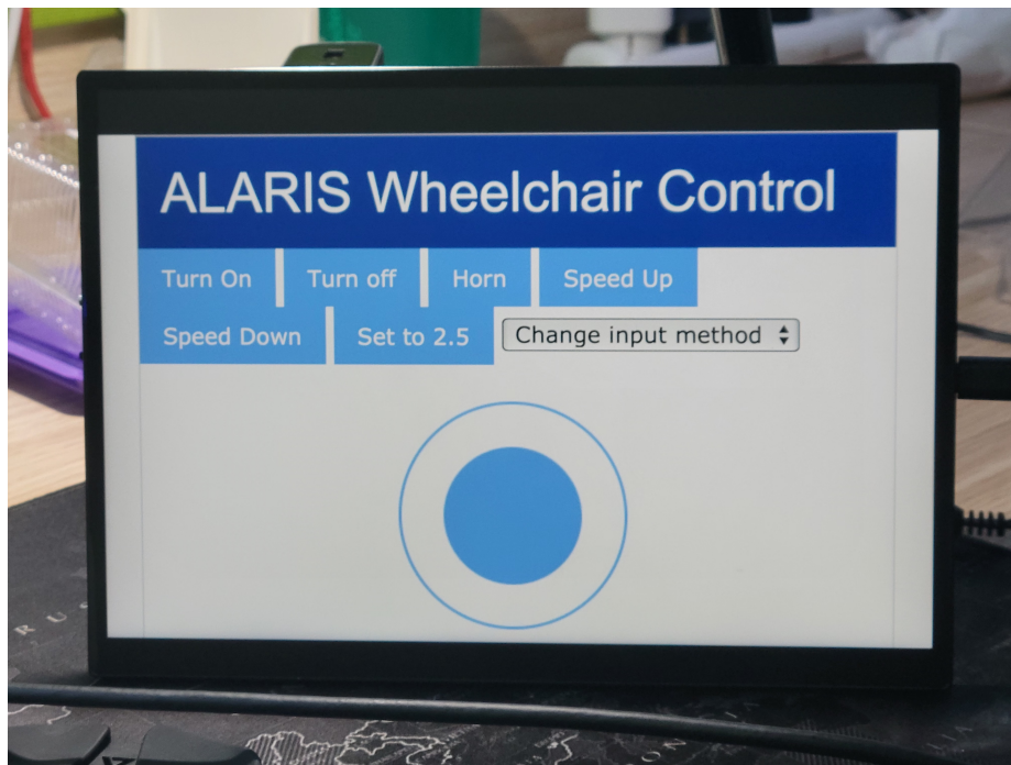
Figure 3-17: External display with a virtual joystick as input
