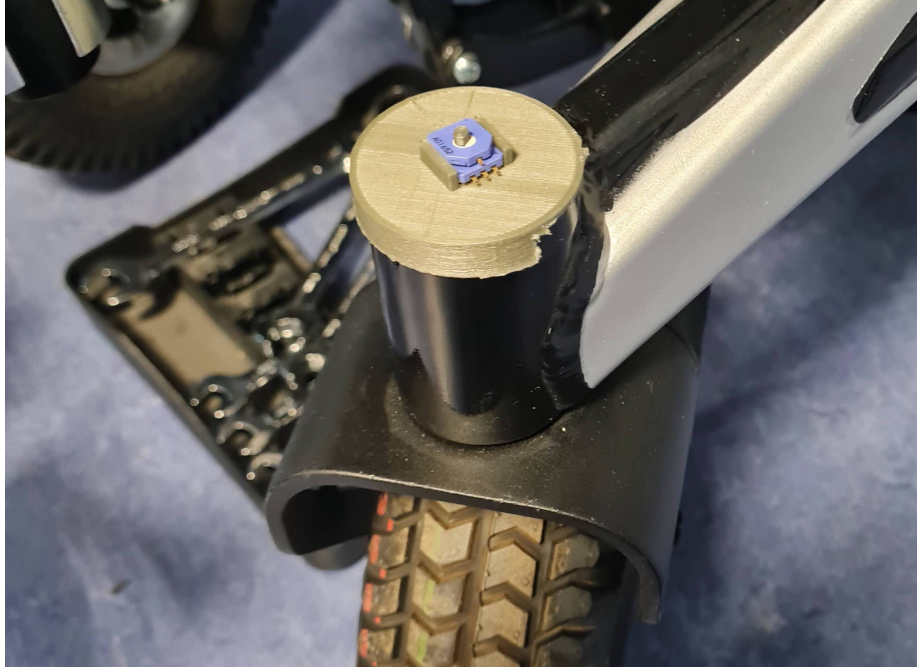
Figure 3-6: Potentiometer on the caster wheel as reference.
