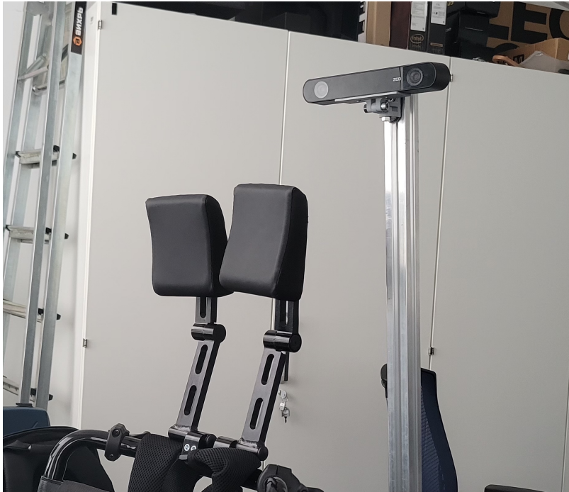
Figure 3-7: ZED2 Camera located on the stand over the head looking down-forward
