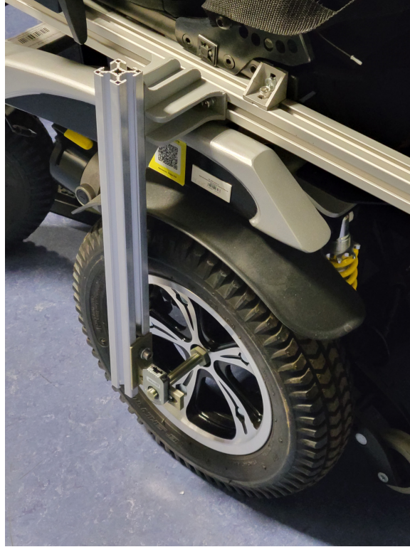
Figure 3-8: Encoder, mounted on the frame, on axis with motor
