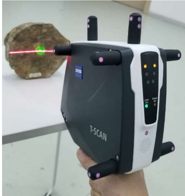
Figure 3.7: ZEISS T-SCAN hand-held line scanner.
