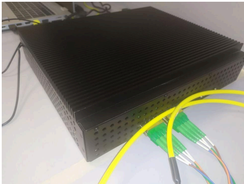
Figure 3.1.2.1: “Hyperion” micron optics device
