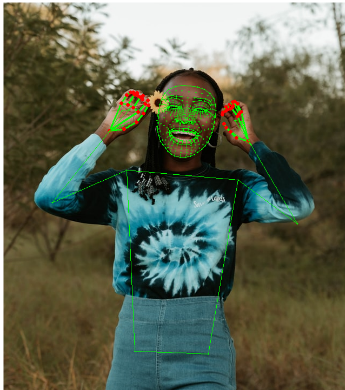
Figure 1-1: Pose, hand, and face keypoint detection using MediaPipe (adapted from [25]).
